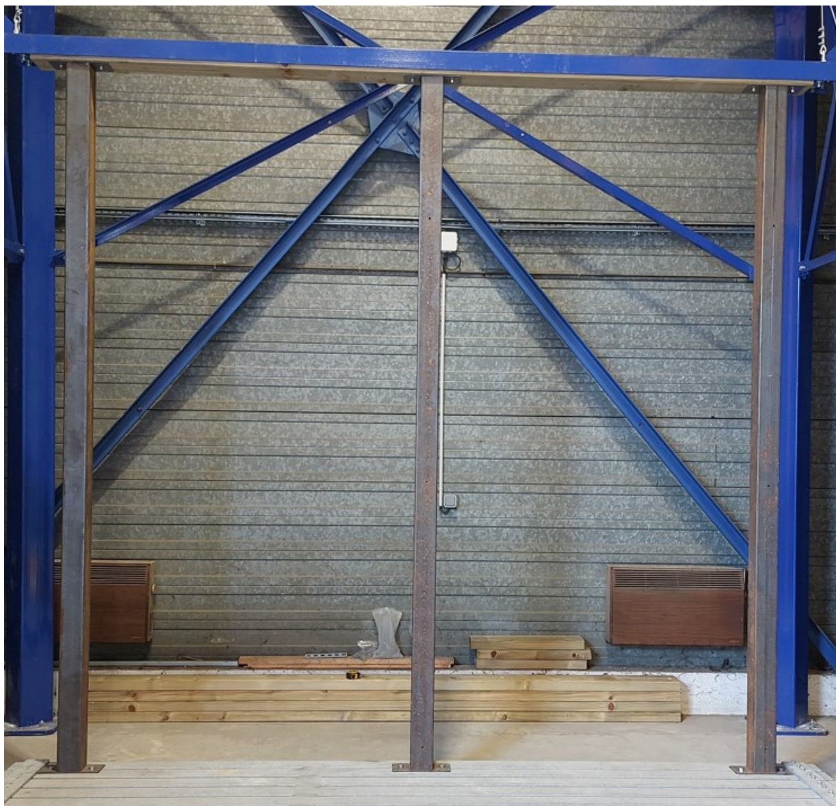
Photo 1 : Structure support tubes aciers creux - LNE
